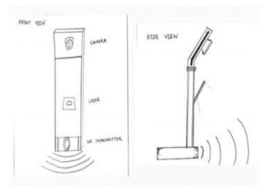
The proposed prototype is shown in the above figure. The left side shows the front view of the device while the right side of the figure shows the side view of the device.
